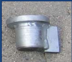
Drive Tool - for installation of the soil postlock.
