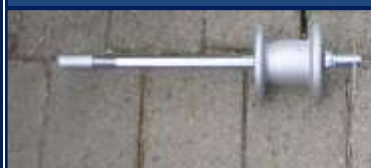
Slide Hammer - for easy wedge removal.
